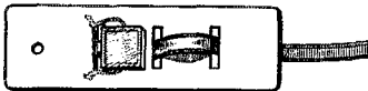
Fig. 1—A sturdy end-insulator for folded dipoles made of Twin-Lead. In addition to providing secure anchorage for the end of the dipole, a convenient mounting place for a fixed mica condenser is available.
