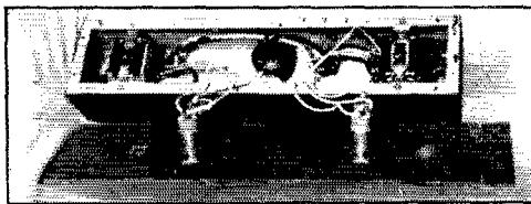
Interior view of the distribution unit, showing the mounting of the plate and filament switches and indicator lamps on the panel.
