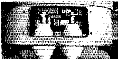
Interior view of rotator showing efficient RF slip rings.
