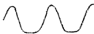
Fig. 5 — Distortion of modulator output waveform which might result if suppressor tube represents lower load impedance than carrier tube (mild overmodulation).
