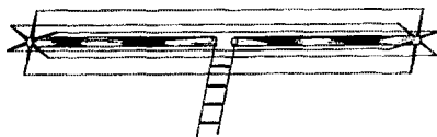
Fig. 1 — Sketch showing the essential plan of constructing a multiclement cage antenna for use as the radiator in a close-spaced array.
