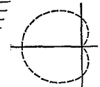
Cardioid (heart-shaped) Polar Pattern. Wide-angle front pick-up, horizontally and vertically, diminishes sharply to dead zone at rear.
