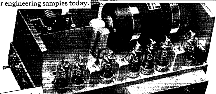
New instant-heating mobile FM transmitter developed by Kaar Engineering Co. uses 7 Hytron 2E25 and 2 Hytron HY69 or HY1269.
