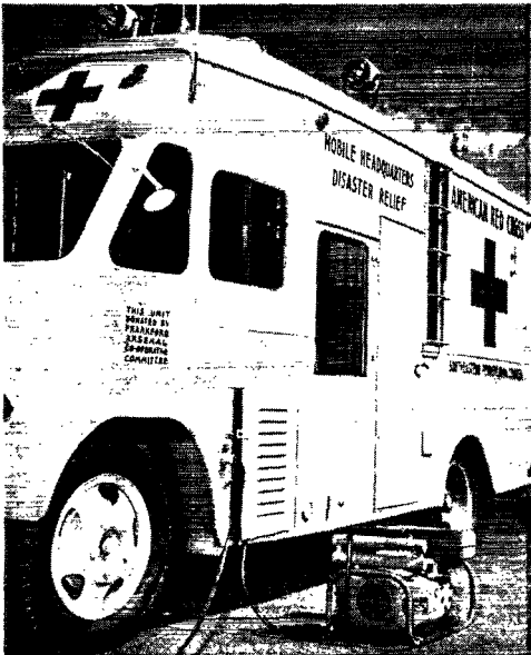
The WERS-equipped mobile disaster unit with its Onan 2-kw. gas-driven 110-volt 60-cycle generator. Note the external connection on the vehicle for the 110-volt power cable.
