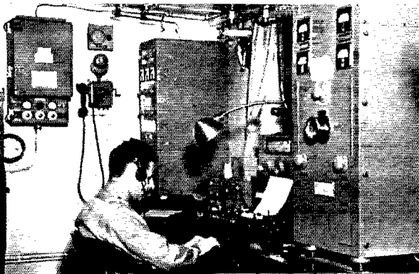
Inside the radio room aboard the Liberty ship. Both side-by-side operating positions are shown in these two views. At the left end of the operating table is the high-frequency transmitter, with the low-frequency transmitter and the emergency set (visible only in the right-hand view) beside it. The auto alarm is on the bulkhead beside the telephone.
