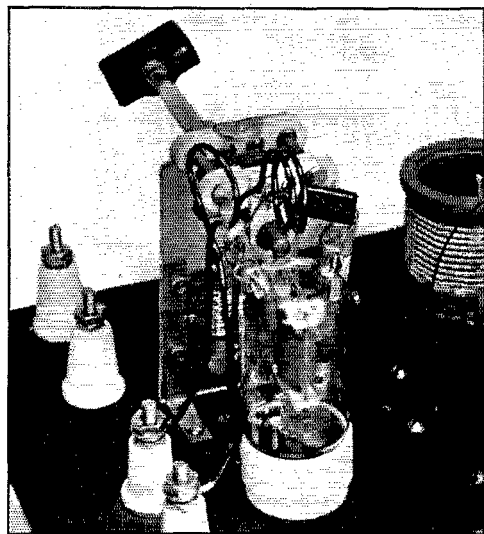
V.h.f. section of the transmitter, showing the arrangement of parts and method of coupling to the antenna.
