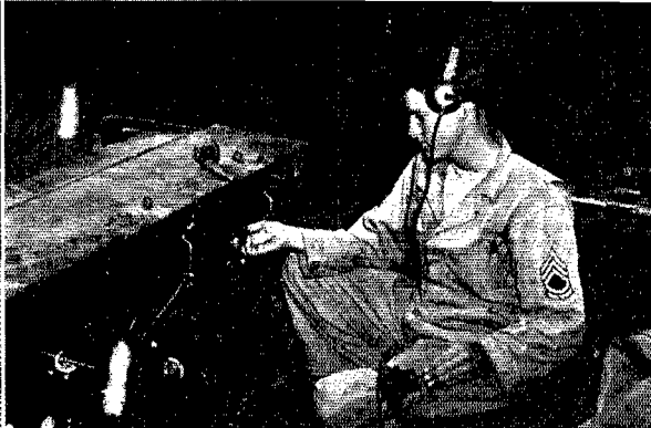
Above — C.w. operator in action, key strapped on leg. A.m. voice may also be used (note microphone).
