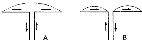
Fig. 2 — The current distribution of a current-fed half-wave element with quarter-wave matching stub is shown at A. At twice the frequency, the current distribution becomes as at B and the system is still very close to resonance, operating as collinear half waves in phase.
