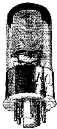
Ceramic base Grounded metal shell
