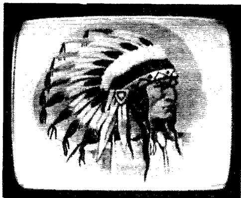
Fig. 6 — This photograph shows the detail that the five-inch electrostatic tube is capable of giving. The picture originated in an r.f. signal generator and was passed through the entire receiver, not just the video circuits alone.
