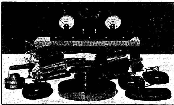
THE SLIP-RINGS, A STRIPPED ARMATURE, AND A REWOUND ONE, SHOWING HOW THE 1/4-INCH DOWELING IS USED TO HOLD WINDINGS IN PLACE, AS WELL AS THE INSULATING PAPER BEFORE BEING TUCKED DOWN AND THE SECURING FIBER STRIPS DRIVEN OVER THEM
