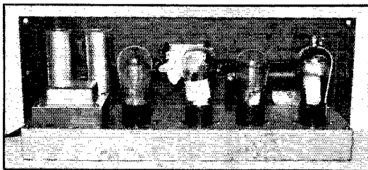
REAR VIEW OF THE UNIT, SHOWING POWER PACK AND RECTIFIER TUBE AT THE LEFT, MULTIVIBRATOR AND SCREEN-GRID OSCILLATOR TUBES TO THE RIGHT
