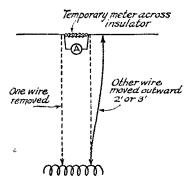
FIG. 5. A METHOD OF FINDING THE WAVE-LENGTH OF THE ANTENNA TOP
