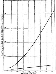
UX 222 SHIELD GRID CONNECTION EFFECT OF CONTROL GRID BIAS ON PLATE CURRENT AND SHIELD GRID CURRENT WHEN PLATE VOLTAGE = +135 AND SHIELD VOLTAGE = +45
