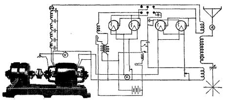
Item 37, 2 unit four bearing set, delivering 1000 volts, 600 watts for plate and 12 volts, 300 watts for filament. The "ESCO" Set is shown here furnishing Power Supply for 4—50 watters in a phone or telegraph set. This is the Item used by CB8 in pioneer achievement of the first two way amateur wireless communication between North and South America.
