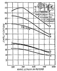
FIG. 3. REPEATER AMPLIFICATION FOR TET-RODES OF SEVERAL TYPES UNDER THE SAME OPERATING CONDITIONS
