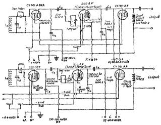
FIG. 3. THE SPACE-CHARGE-TYPE A.F. AMPLIFIER USED WITH DIFFERENT DETECTORS
