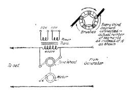
brushes make contact on the commutator, which has every third sogment connected together. The brushes are adjusted to make contact to any two of the segments that are connected. This would, when the motor was running, give us an interrupted circuit with a frequency of about 360 interruptions per second.
