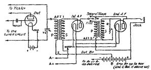
FIG. 1. A TWO-STAGE AUDIO AMPLIFIER WITH RESIST-ANCE CONTROL OF AMPLIFICATION AT THE INPUT OF THE SECOND TUBE, ALSO SWITCHING ARRANGEMENT FOR CUTTING OFF THE 2ND STAGE
