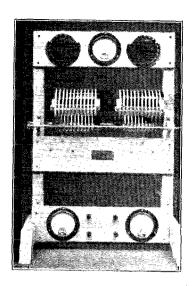
The main transmitter of the University of Michigan, Greenland Expedition. A ½KW tube is used in a Reinartz circuit at nxIXL. This type of mounting with a couple of back braces works nicely with any circuit. nxIXL works on 25, 35, and 45 meters wavelength.
