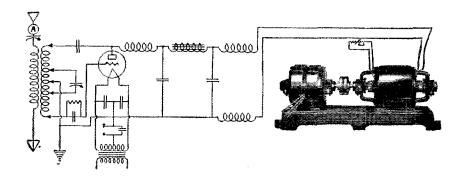
This is Item #26 used as a Plate Power Supply for a 204-A Tube.
