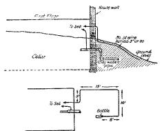
FIG. 3. THE ARRANGEMENT USED FOR RECEPTION AT 5VU, STATION OF CECIL PATTERSON AT FROST, TEXAS—WHERE THERE IS STATIC
