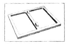
sults. Your troubles are materially reduced though, if you are able to get some sort of a skeleton frame to start with. The illustration shows a cast aluminum frame that should prove of great help.
