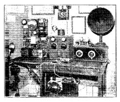
5SI-A REAL RM LAYOUT Note dynamotor at bottom, which furnished emerg-ency plate supply during the Mississippi flood.
