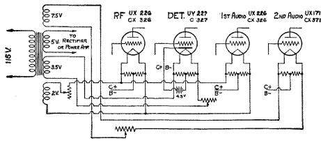
For the past several seasons the trend has been toward complete battery elimination. Many satisfactory plate supply units operating from A. C. have been developed but filament operation from an A. C. source has presented more of a problem due to the larger currents required and increased expense in the rectifier and filter circuits.
