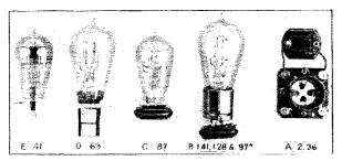
GROUP OF SHORT-WAVE ULTRAUDION OSCILLATORS SHOWING CONSTRUCTION NEEDED WHEN OPERATING AT 34 M. DIRECTLY AND ADVANTAGE OF WORKING IN MANNER SUGGESTED. THIS IS THE GROUP MENTIONED BEFORE AS USED BY PHELPS AT 2EB.
