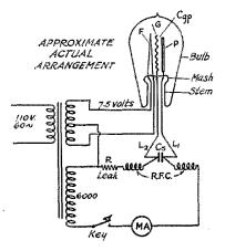
FIG. I THE ULTRAUDION CIRCUIT USED, SHOWING SCHEMATIC AND ACTUAL FORMS
