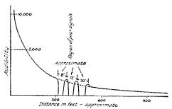
FIG. 5 CURVE SHOWING APPROXIMATE MANNER IN WHICH LOW-POWER %-METER SIGNAL VARIED IN AUDIBILITY WHEN RECEIVER WAS MOVED AWAY FROM STATION
