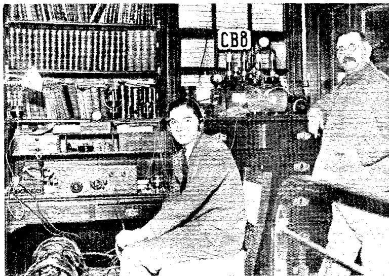
A NEW PICTURE OF CBS Here are the Messrs. Braggio at their station at Bernal, near Buenos Aires, the only South American station to be heard in North America during the tests. Our hunch about their transmitter was wrong—they have a new one using four UV-203-A's working into a beautiful vertical cage aerial a hundred feet high.
