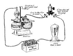
connected in series with the battery and the voltage of the battery being charged. For charging a 45-volt battery a 75-watt lamp can be used. It will light at about half brilliancy when charging.
