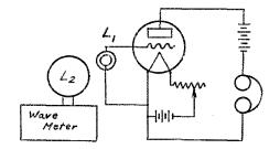
FIG. 17—TUNING THE R.F. COILS
