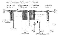
Fig. 23-The Tuner at 9ZT-XAX.
