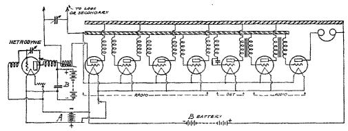
Fig. 14-Circuit of the Kimball Superheterodyne
