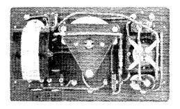
the two fixed condensers that are used for different wavelength ranges. The variable condenser and condenser switch are mounted near the center of the panel.
