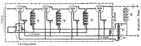
Fig. 2-General Circuit For Air-Core Transformers (Ballantine)
