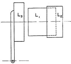
Arrangement of Heterodyne and Pickup Coils
