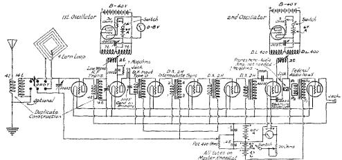
FIG. 22-CONNECTIONS OF THE "C.W." SUPERHETERODYNE AT 3XAQ.
