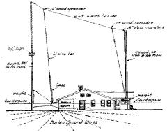
FIG. 4 THE ANTENNA AT 9ZT
