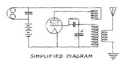
for the tickler is made of a 3" bakelite tube with most of the tube cut away, leaving a skeleton. The winding is in two sections, 11 turns on one side of the shaft and 12 turns on the other side. The turns in each section are placed close together.
