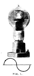
TUBE JUST BEGINNING TO CONDUCT FORWARD DIRECTION
