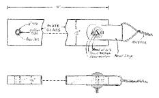
FIG 6 18' GLASS INSULATORS USED AT 9ZT
