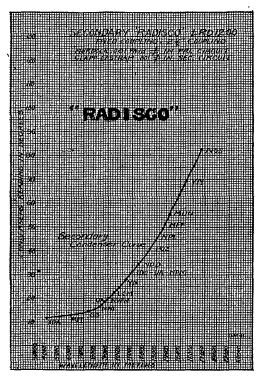
THE CURVE on the left shows the performance of RADISCO inductances at an amateur station located near Boston. In two hours time the stations noted were received—and using but one vacuum tube. The antenna used was 50' in length and 40' in height.
