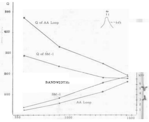
From the passband figure it is obvious that both antennas have high enough Q on the bottom of the band to cut sidebands by a significant amount; the lack of a Q control on the SM-1 is thus a real disadvantage.
