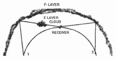
Figure 1. Sporadic E Layer clouds can cause interruption of F Layer propagation paths.
