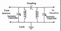
Figure 1: A resonant preselector provides front end selectivity and a static discharge path to ground to protect your expensive receiver. Its loss is greater than the Transmatch.
