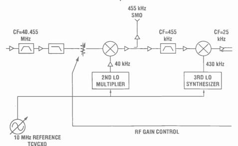
Figure 8. The HF-1000 converts the signal down to a 25 kHz center frequency that the digital circuits in the DSP function can convert to a series of numbers for computer processing
