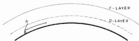
Figure 3a—1. Daytime. Skywave signals for MW stations are absorbed in the "D" region at Point A. Long distance propagation proceeds by groundwave only and signals are steady.
