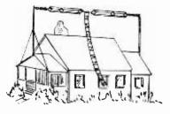
Fig. 1—Cage Doublet Antenna (886 or 862), for limited space; lead-in off center.
