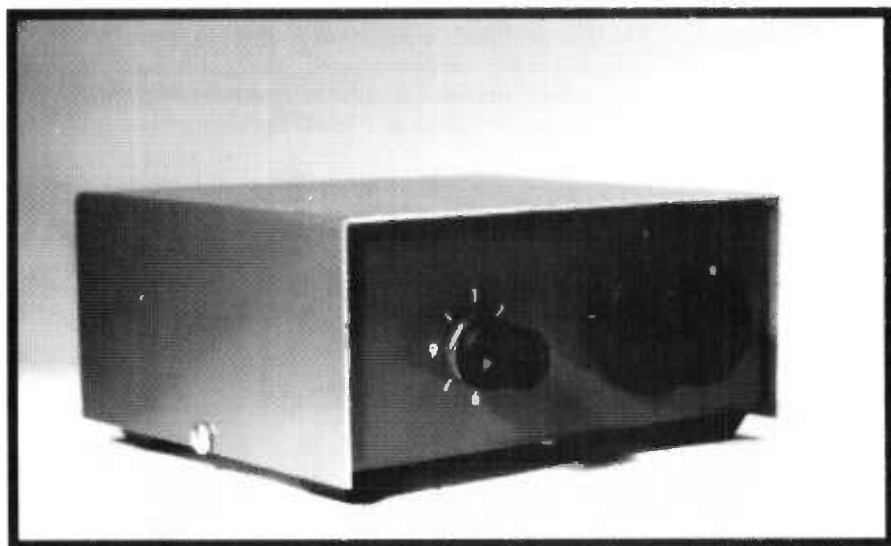
Opposite Page (top): Hambrew-built 30 Meter Ramsey transmitter kit with power meter added from used CB rig.
