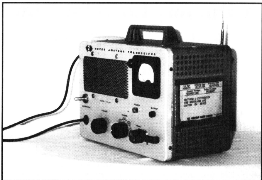
The license is held on the side of the box. An internal LED glows to give the illusion of hot tubes.
