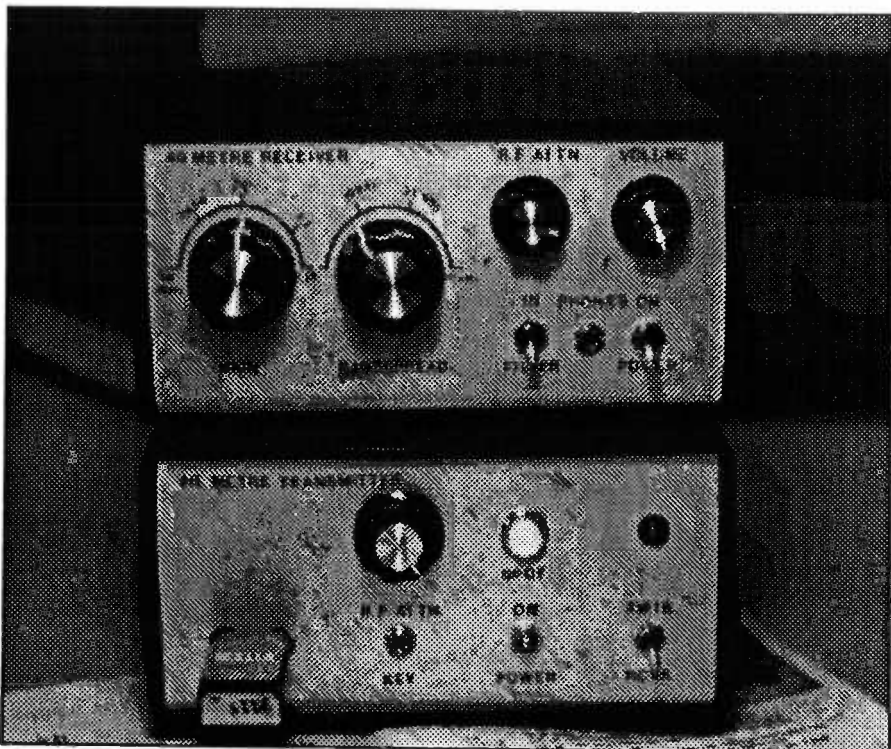
Very nice work! Built by VE3GQD, Reg Tremblay. Top photo shows the K6EIL Receiver with bandspread sitting on top of the NG7D Two'er III Salvation Xmtr (Spring, '94 HB) (both photos: VE3GQD)
