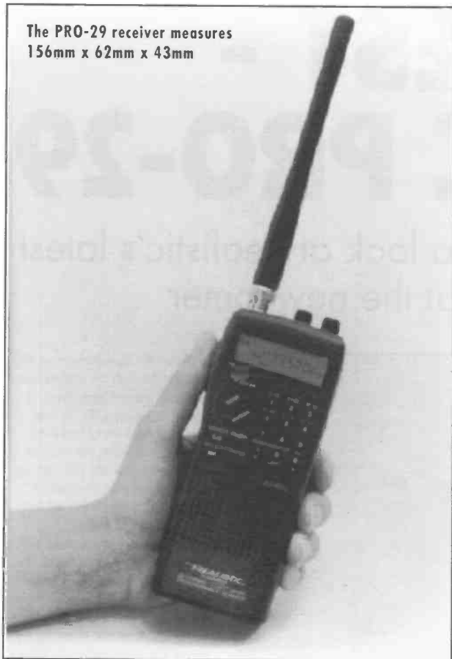
An internal charging circuit lets you charge nicads from an external DC supply or an AC adapter through the side-mounted 'charger' jack.
