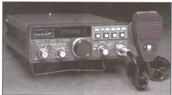
Sid recently bought a second hand FT-480, he said that after he'd fully installed it, the output had dropped to just under 5W, whereas it should have been 10-12W
