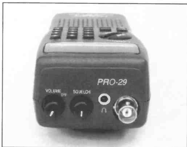
A 3.5mm jack socket is fitted to the top panel, which lets you plug in an optional earphone for private listening or an external amplified speaker for a greater audio level.
