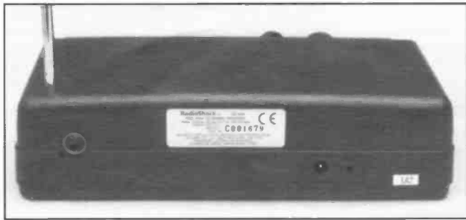
An external aerial can be plugged in, although the connector for this is a 'car radio' type coax socket
