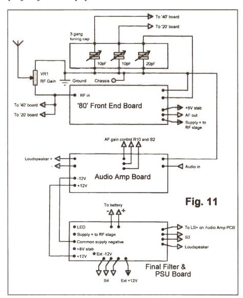
Block diagram showiing earth returns and common supply negative connection. Band switching and associated wiring not shown.
