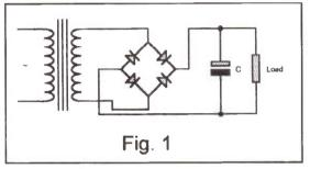
Fig. 1 - A simplistic view of the action of the reservoir capacitor C in a DC power supply
