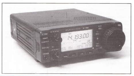
graphically reduces when you switch this in. A switchable preamp, attenuator, and an RF gain control (which sometimes isn't found on such small sets!) plus a pulse-type noise blanker add to the QRM-fighting measures. Besides the 2.3kHz, 6kHz (AM) and 8/15kHz (FM) filter bandwidths fitted as standard, optional filters of 1.9kHz and 2.8kHz are available for SSB, RTTY and CW, and 250Hz and 500Hz for CW/RTTY.
