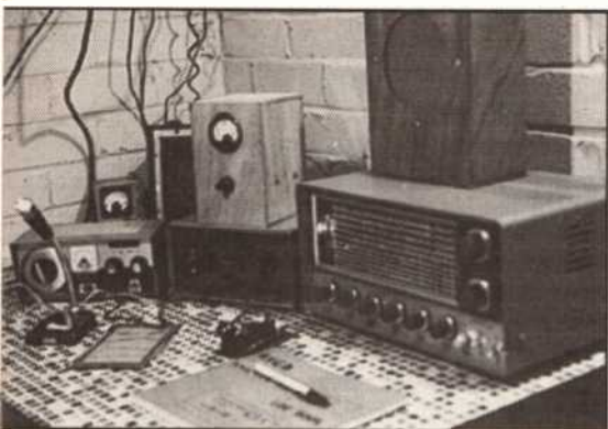
The G3XTT station of 1968, 10W into a Codar AT5 made CW a necessity!
