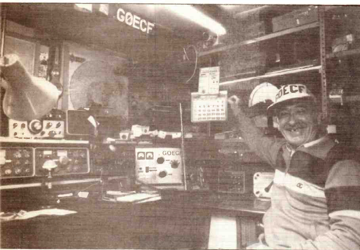
Vico GOECF in his shack. The steering wheel for the rotatable quad is just by his right hand.
