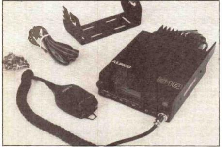
and the often-used 1750Hz repeater Tone and channel Scan buttons were sensibly located for quick operation by feel alone. The receiver volume, squelch and main tuning knobs were sensibly positioned, although I found the microphone Up/Down buttons easier when attempting a QSY.
