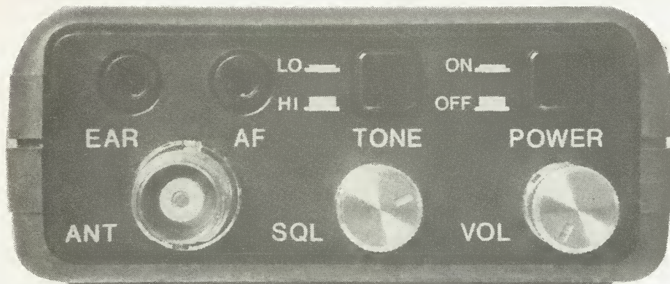
Top panel detail — the push-on push-off power button can be knocked 'on' by mistake.
