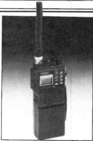
The new £250 Yaesu FT23 handie, 2 to 5W (depending on battery pack option). Die-cast case and rain-proof construction.
