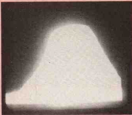
The transmitter bandwidth with the centre on 50MHz, same scales as before.
