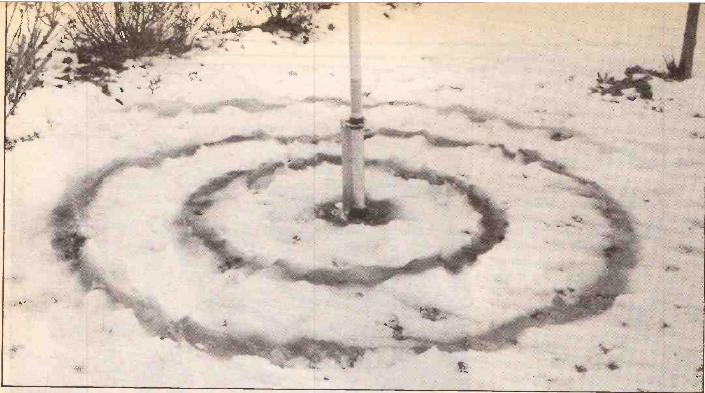
RF burns can occur on surrounding ground around long standing high power aerials. The RF can completely sterilise the ground. The rings are proportional to the frequency operated on.
