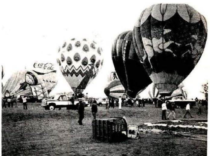
A part of the balloon-ride scene is getting that giant bag ready for lift-off, and sometimes it takes all hands to keep it under control. Here's WB6NOA performing double duty, upper left, by communicating as well as holding the fabric up for a preliminary air fill. A fan forces air into the balloon, then the burner is lighted to provide some heat for lift. This balancing act continues until there is enough lift to keep everything upright, then there's a last-minute scramble to get everyone aboard.
