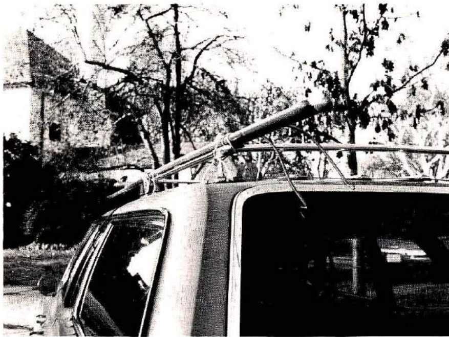
Two Bean Poles ride easily on the car-top carrier when you are traveling. The board and coaxial cable are carried inside but can be assembled in a few moments when you arrive at your destination.
