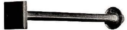
Feedthrough tube for bringing coaxial cable into a building. The metal bracket should be grounded using a length of no. 10 (2.6 mm) or larger wire to a ground rod.
