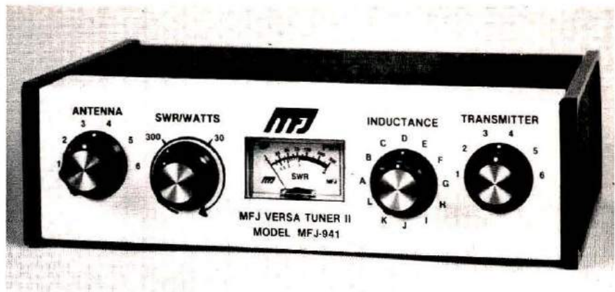
The MFJ Versa Tuner II covers the frequency range from 1.8 to 30 MHz and will match antennas fed with coaxial cable, open-wire line or twinlead, or a random wire. The tuner features a built-in SWR meter and dual-range wattmeter (30 to 300 watts full scale), as well as an antenna selection switch (photo courtesy MFJ Electronics).
