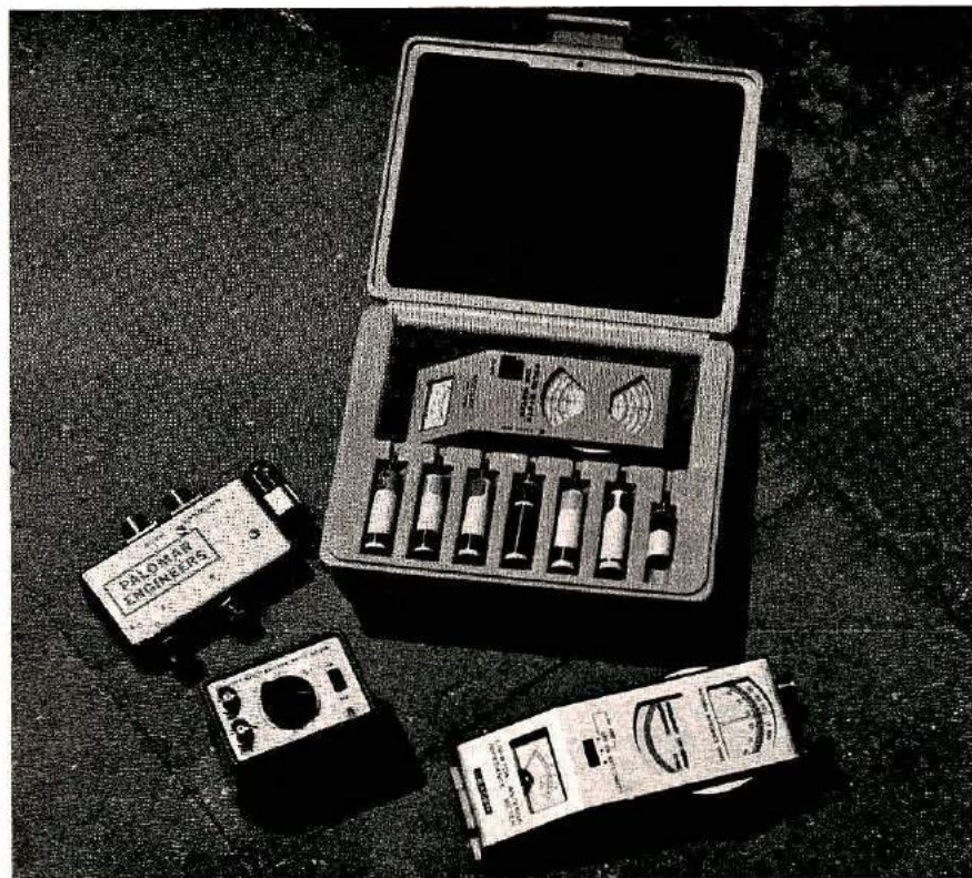
Fig. 3. Antenna test equipment: (left to right) Palomar Engineers R-X noise bridge, Omega-T noise bridge, Heath dip oscillator, and a Leader impedance bridge.
