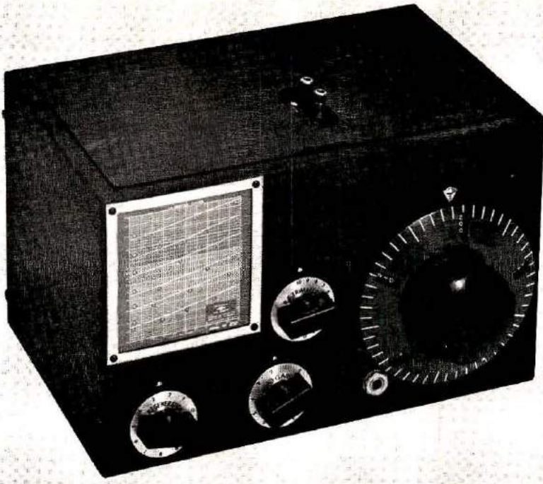
The National 1-10 vhf/uhf receiver, first introduced in 1936, tuned from 30 to 300 MHz and covered the 5-meter, 2-1/2-meter, and 1-1/4-meter bands then available to amateurs. This popular receiver featured an rf amplifier stage followed by a superregenerative detector and two stages of audio.
