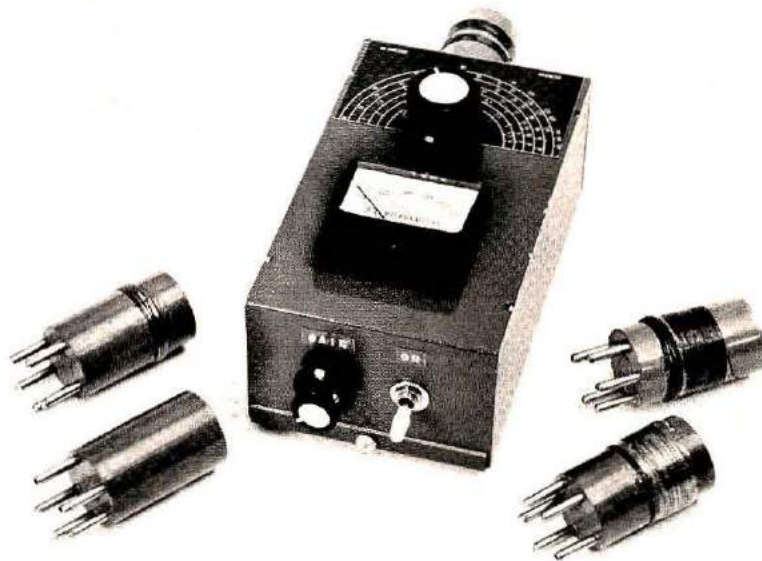
The wavemeter could be one of the most useful items around your radio room. Here one coil is plugged into the socket at the top of the meter box. The "bare" coil form shown to the left has the 60 to 130-MHz coil inside it. A hairpin loop for the highest-frequency range is shown in Fig. 8.
