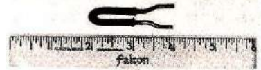
Fig. 8. The "coil" for the highest-frequency range could be described as a hairpin. It can be made to the correct size by comparing it to the rule. Bare ends of the heavy wire plug directly into the socket on the wavemeter.
