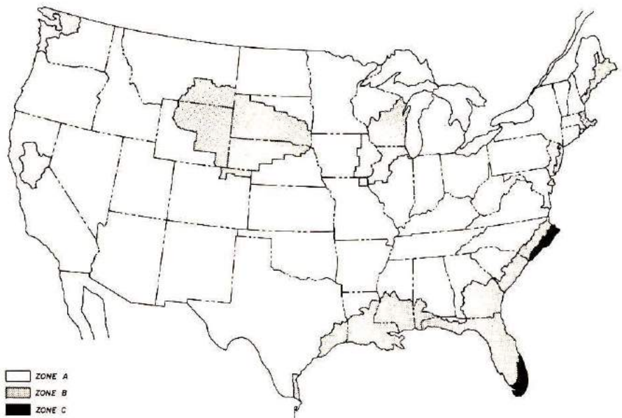
Fig. 1. Expected wind loading areas of the United States from EIA Standard RS-222-B. Zone A includes wind velocities to 86.6 mph (139.5 km/h) or 30 pounds per square foot (1.44 kilopascals [kPa]) of impact pressure. Zone B is up to 100 mph (161 km/h) or 40 pounds per square foot (1.92 kPa). Zone C is rated at 111.8 mph (180 km/h) or 50 pounds per square foot (2.39 kPa). This information is for towers which are less than 300 feet (91m) high.
