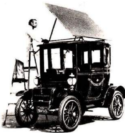
Old vehicle meets new power source — a 1912 Baker Electric horseless carriage was fitted out with a solar panel by International Rectifier as part of their research and demonstration program. The 10640 individual cells provide a combined power output of approximately 200 watts to recharge the vehicle's batteries. The 12 batteries and 3-horsepower motor give the Baker a range of approximately 80 km (50 miles) and a top speed of 32 km/hr (20 mph) (photo courtesy International Rectifier Corporation).
