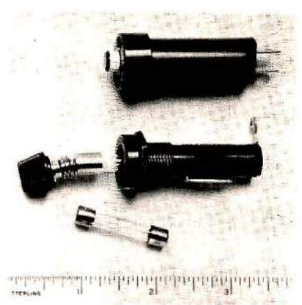
The Heinemann Electric Re-Cirk-It (top) protects electronic circuitry like a fuse (bottom), but can be reset. It is designed to be installed in the same panel space as a conventional fuseholder. The Re-Cirk-It is available with current ratings from 0.25 through 10 amperes (photo courtesy Heinemann Electric Company).
