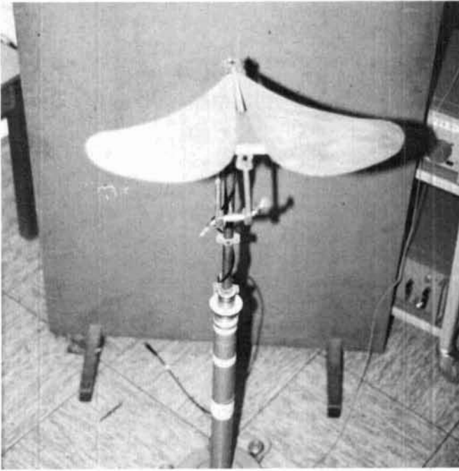
Common materials can be used to build the antenna. Here you see the Heart antenna made of aluminum sheet stock.
