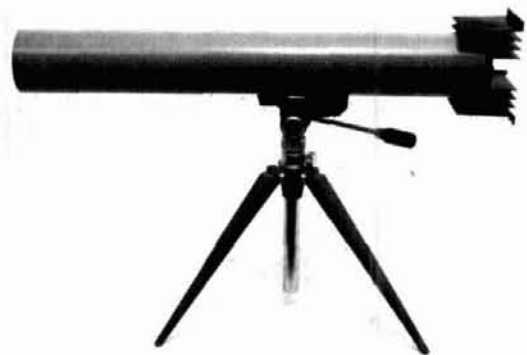
Photo C. This helium Neon laser is housed in a 2½-inch diameter PVC pipe, which also contains a commercial 12-volt inverter power supply.
