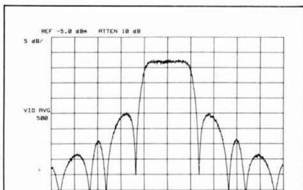
fig. 19. Continuous phase FSK, 190 Hz shift 300 Baud ASCII equivalent.
