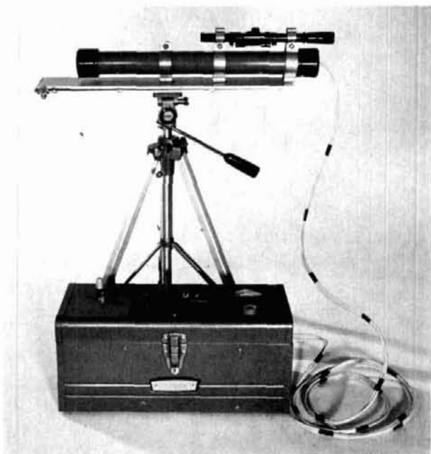
Photo B. This Helium Neon laser uses the power supply circuit shown in fig. 7. Power supply and battery are housed in a tool box.
