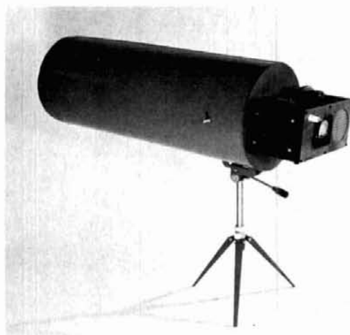
Photo G. Portable laser communications receiver uses a 10-inch diameter Fresnel lens for the "antenna" and 931A photomultiplier tube as the detector.
