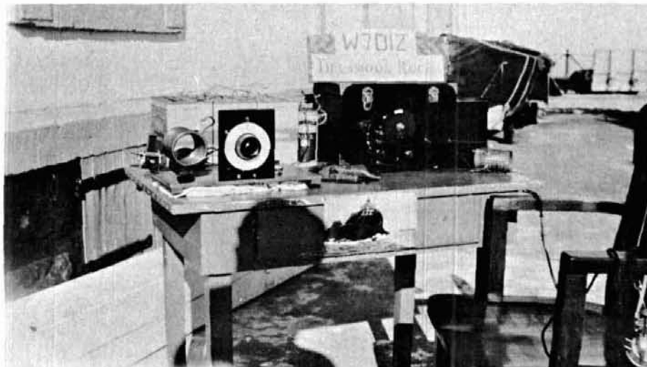
Photo A. After the terrible storm, W7DIZ rebuilt his "junk box" radio station. At left is the one-tube transmitter, with the copper tubing tank coil. In the center, in front of the tool box, is the one-tube receiver. A heavy brass hand key is positioned on the table near the transmitter. With this simple, home-made equipment, W7DIZ maintained schedules and kept the Tillamook light on the air, in the ham bands.
