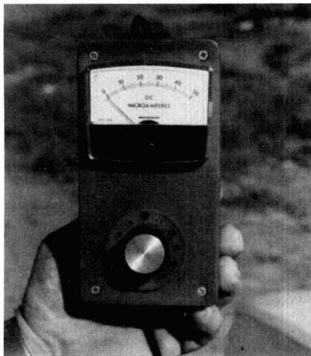
Photo 1. The K1ZJH Fox Box external metering and attenuator control box.
