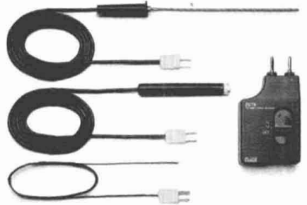
Surface, immersion and general-purpose probes with "mini" thermocouple connectors are available for the Fluke 80TK.
