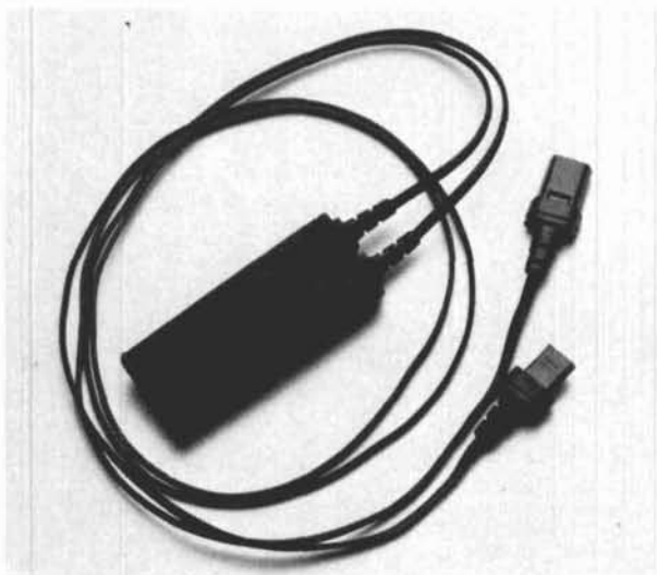
fig. 4. The HP-41 can be safely linked to the HP-IL by using the HP82160A module.
