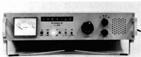
fig. 2. Photograph of a semi-synthesized 2-meter transceiver using the converter shown in fig. 1.
