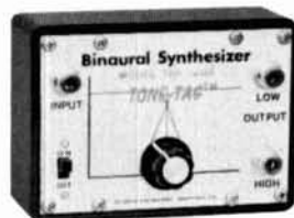
Model 700 - 7 IC op amps, 6 diodes on 2 PC boards 2 7/8 X 4 X 2 inches deep
