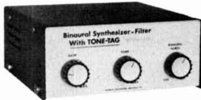
Model 1100 - 13 IC op amps, 4 transistors, 10 diodes on 4 PC boards. 3 X 6 3/8 X 8 inches deep
