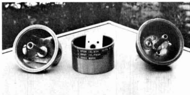
Interior view of top and bottom end bells. At left is the interior of the top end bell integral (soldered) with the upper half of the pop-up stem center conductor. The center is the Teflon block table leaning on the wall of the central brass shell of the instrument. Right shows the interior of the bottom end bell with the jack ends of the banana-plug and jack primary-coil connectors. Note window of large end of pop-up stem to accommodate jumper wire (with sleeving) from coax center conductor to insulated banana-plug/jack. The lower plug/jack is grounded to the cup bottom.
