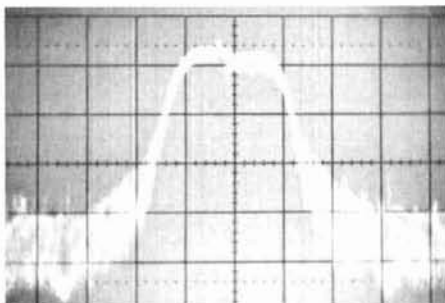
fig. 28. TV station. BW 250 kHz, Scan 100 kHz/division. Adjust frequency control to the video carrier of any TV station between channel 2 and channel 6. Connect 50- or 75-ohm TV antenna to input. Line lock the scope and note video sidebands and vertical sync pulse, which will drift through the top of the signal.
