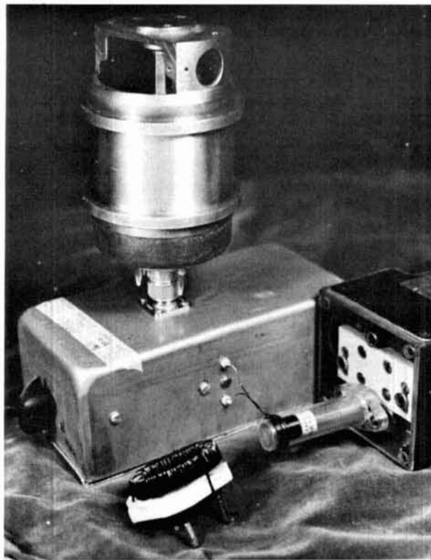
Selsyn-case cup permeability meter in place on a support fixture, which also supports the grid-dip oscillator link. Knob on the fixture varies the loop capacitor, C . The grid-dip oscillator is next to and slightly to the rear of the support fixture. The toroid primary coil is in the foreground. It is laced to Teflon-sheet padding on a Teflon base. Banana plugs allow coil to be plugged into bottom of cup. The coil consists of 100 turns of no. 24 AWG (0.5mm) wire on an Arnold Engineering type AM-12 core (core no. 10 in table 1).
