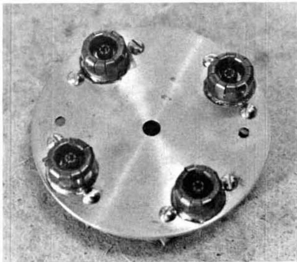
Completed cathode disk showing the filament and cathode connections.
