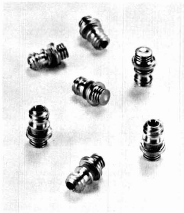
Construction of Gunn diodes. Most of the package shown here is actually the heatsink — the ceramic-packaged device is only 0.025" (0.6mm) thick. To give you an idea of size, the stud is threaded 3-48 (M2.5).
