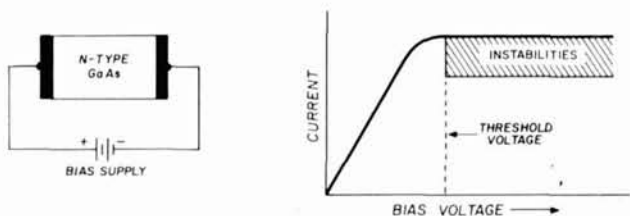
fig. 9. When the bias voltage across a sample of n-type gallium arsenide (GaAs) is increased above the threshold point, the current becomes unstable and pulsates in a cyclic way. This is a result of negative resistance and is called the Gunn effect.
