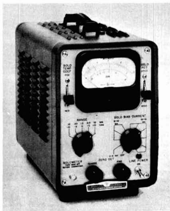
The Hewlett-Packard model 430C Microwave Power Meter is commonly available on the surplus market at reasonable prices. It may be used with either a thermistor or a barretter mount.
