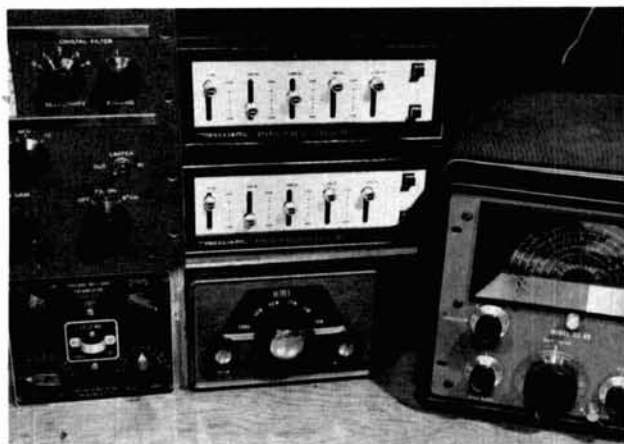
The Stereo Frequency Equalizer can be used to shape the audio output of most receivers. They will provide attenuation or emphasis of specific frequency segments.
