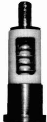
TRAPATT diode configuration built by RCA in 1970 that provided 1200 watts peak power output at 1100 MHz with about 25% efficiency. Five TRAPATT diodes are stacked in a 1N23 rectifier package.
