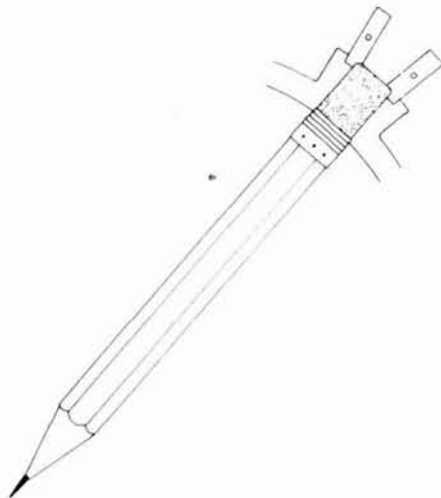
fig. 3. Be sure to clean the portion of the switch wiper contact surface that is underneath the fixed contacts. This can be done by rotating the switch while holding the eraser between two contacts.
